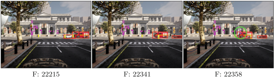
Fig. 7. A series of matching frames with object detections within the CARLA simulator where a vehicle (red) eventually occludes a traffic sign (pink) in the green circle. (Color figure online)
